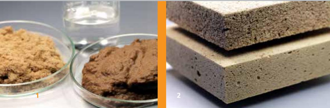
**1** Starting material for wood foam: wood fibers and water are ground to a suspension and foamed.
