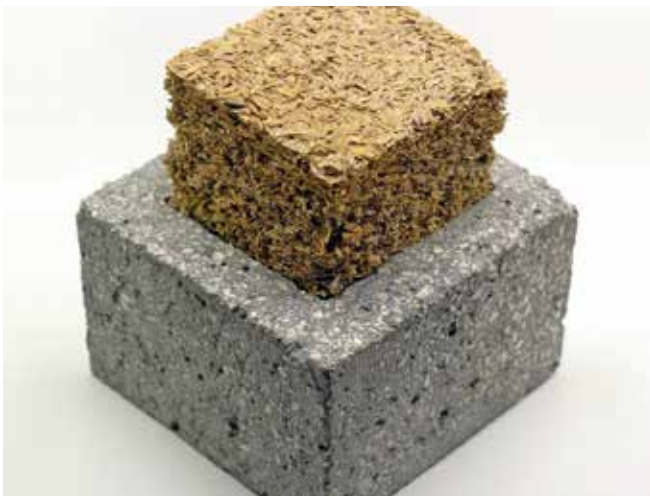
Concrete component made of recycled aggregates and rice-husk ash with rice-straw insulation.
