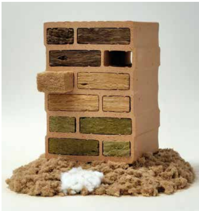
Brick filled with various insulation materials, including a mixture of beech and bicomponent fibers.
