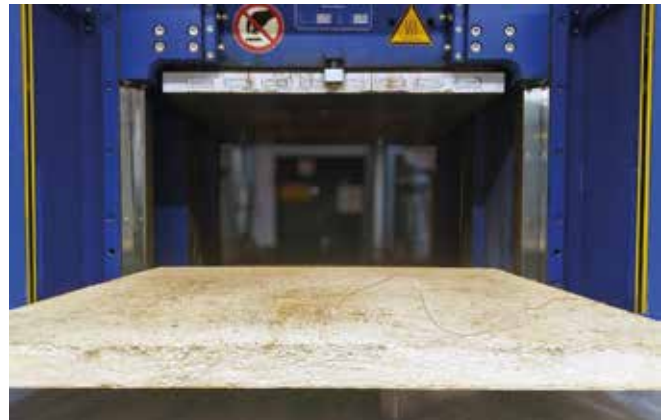
Freshly pressed! Mycelium-based thermal-insulation panel with optimized properties after heat-pressing step.
