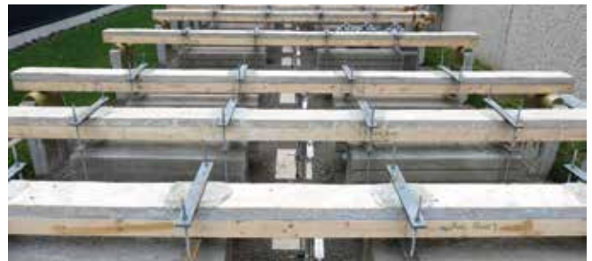
Adhesively bonded wood-concrete and wood-fiber-reinforced polymer (FRP) composite panels subjected to sustained bending loads under outdoor environmental conditions.
