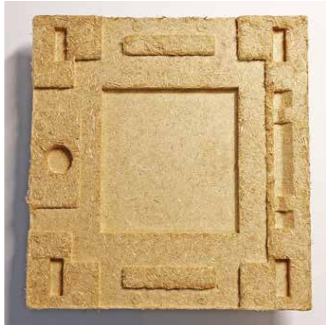
Molded part consisting of recycled balsa wood and bicomponent fibers made from PE/PP.
