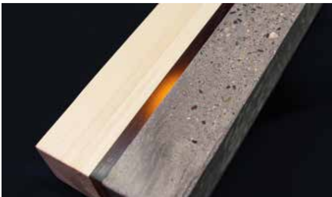
Bonded wood-concrete-composite shear-test specimen.
