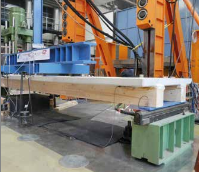
Fig. Load-bearing timber-concrete composite elements with long span ranges (here: 6.15 m).
