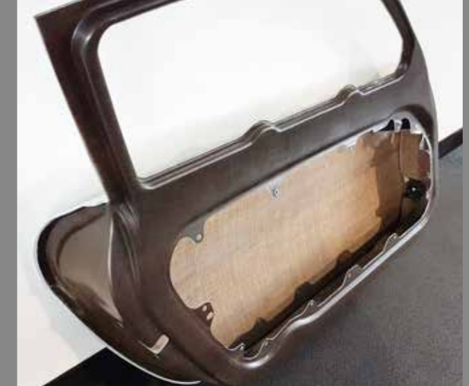
Fig. Vehicle door made from natural-fiber-reinforced plastic (NFRP).
