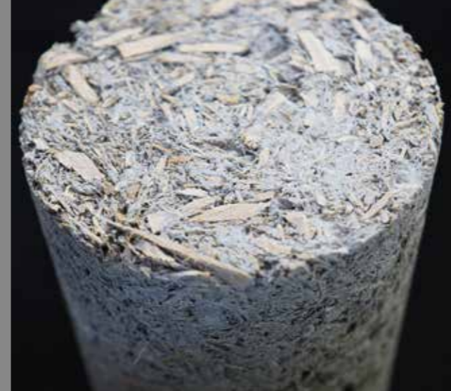
Fig. Test specimen made from a wood-concrete hybrid material.
