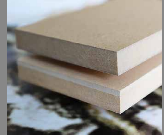
Fig. Medium-density wood-fiber boards with a proportion of beet pellets.
