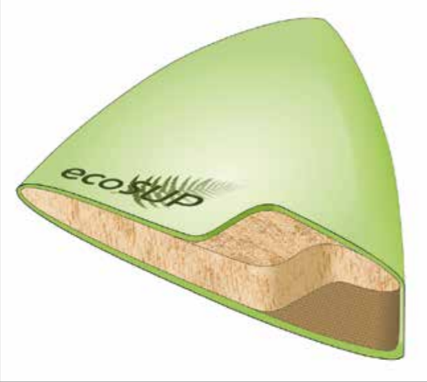
Fig. The cross-section of the paddleboard shows the sandwich construction: core made from recycled balsa wood with an outer shell of natural-fiber-reinforced bioplastics.
